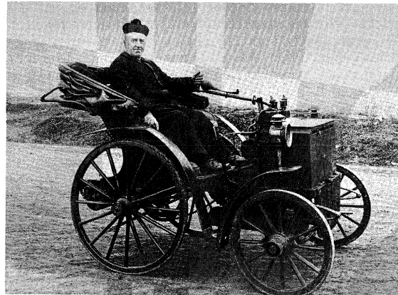
Figure 4: Panhard-Levassor, 1891, the first vehicle with an internal-combustion engine mounted at the front of the chassis.
