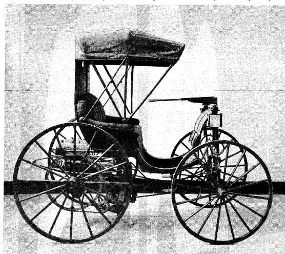
Figure 6: Duryea, 1893, a one-cylinder gasoline engine with electrical ignition.
