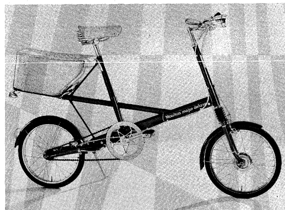
Figure 2: (Top) Modern diamond-frame touring bicycle. (Bottom) Small-wheeled Moulton cross-frame bicycle with patented suspension.
